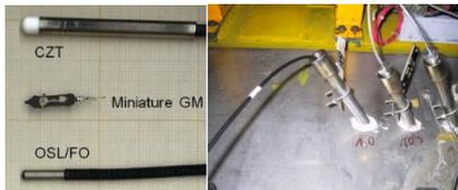
Figure 1: Left - view of the OSL/FO sensor and view of GM and CZT devices for comparison
